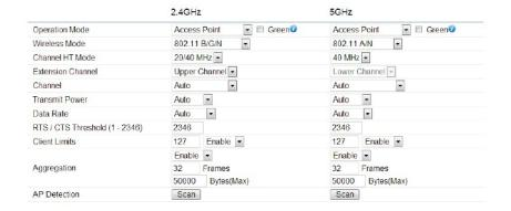
**Data Rate:** Select a data rate from the drop-down list. The data rate affects throughput of data in the EAP1750H. The lower the data rate, the lower the throughput, though transmission distance will be lowered as well.
