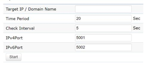
**Target IP / Domain Name:** Enter an IP address or domain name you wish to impelement a speed test for realizing the variance on wireless speed.
