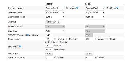
**Operation Mode:** Scrow down this list to select operation modes for implementing on this radio. The default operation mode is **Access Point** on base stations and Access Points and is **Client Bridge** on Client Premise Equipements (CPE). Meanwhile, EnGenius outdoor devices also support WDS modes for peer to peer or peer to multi-peer connections.
